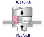
Press Fastener Into Sheet / Panel Until The Knurled Section Under The Head Is No Longer Visable
